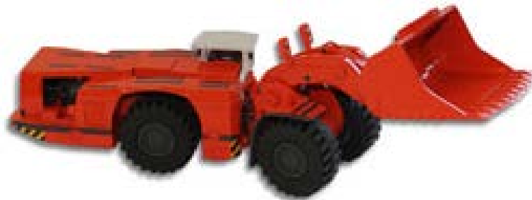
Fig. 2. Overview of the machine for loading, transportation and storage, TORO 151 model manufactured by Sandvik company
